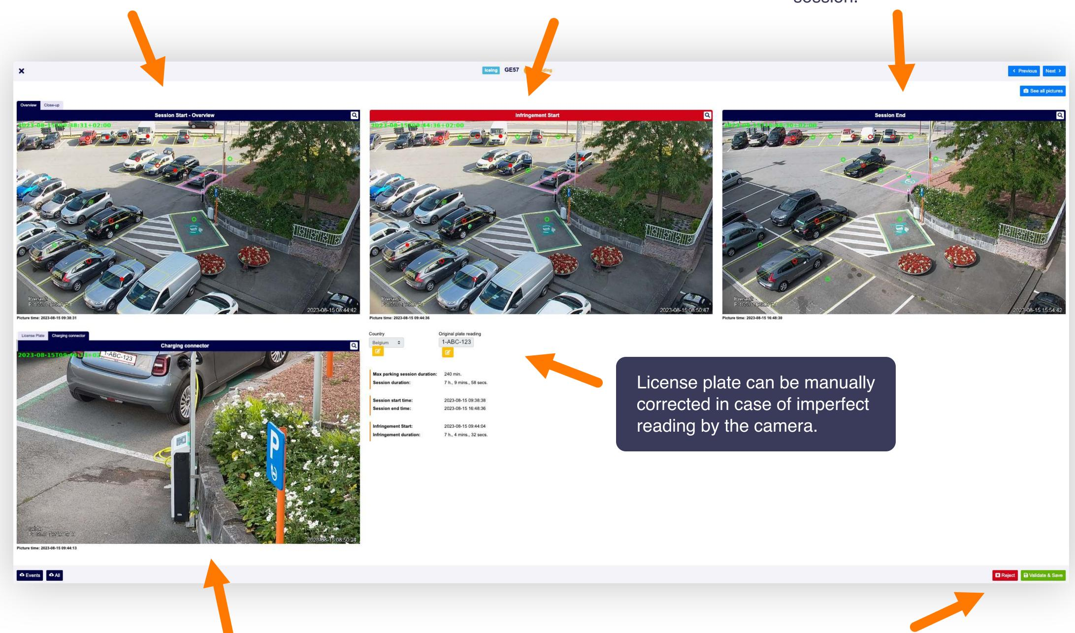
Camera zooms in on the car at the start of infraction and capturing a close-up image of the license plate as evidence. In case of EV close up, an additional picture of charger status (showing cable connected or not, LED) is stored as supplementary evidence.
